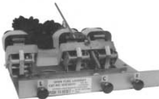
Figure 3U: Open Fuse Lock-Out Device (OFLO)–(Ref. 27)
