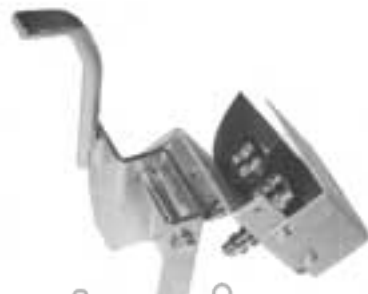
Figure 3S: Cut-Off Switch Assembly (Ref. 14)
