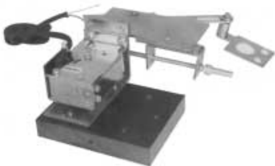
Figure 3T: Flux Shift Trip Device (Ref. 17)
